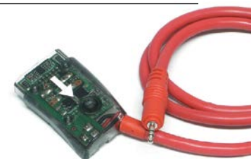
SCP01c Analog Common Positive (Negative Wiring) Cartridge
