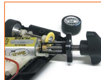
Pull the pinion leaving motor and crown in place
