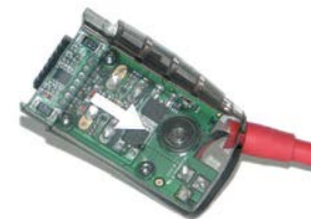
SCP01b Analog Common Ground (Positive Wiring) Cartridge
