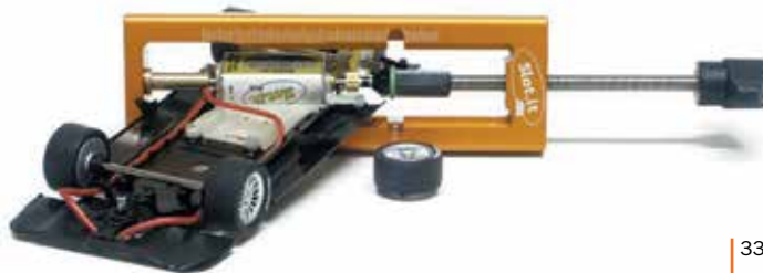
Push the pinion leaving motor and crown in place
