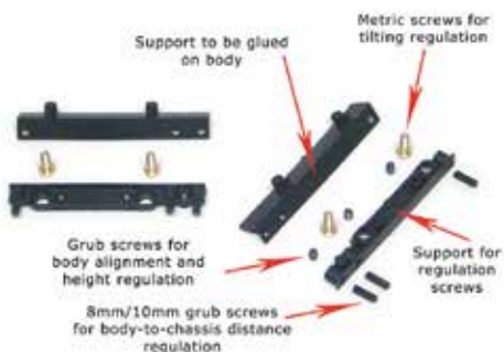
CH57b Body-to-chassis HRS2 adapter
